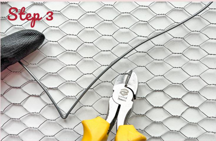
Cut around the shape using wire cutters. It's best to leave approximately 2 centimetres of chicken wire on the sides.
