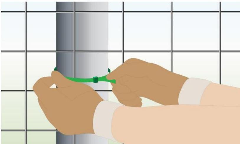
**Step 2: Tighten the Cable Tie**
