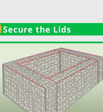
To prevent any movement, secure the adjoining corners of the baskets at both the top and bottom with a piece of tying wire.
