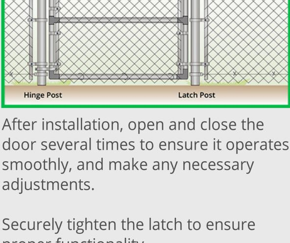
Place a brace across the center of the frame to prevent the sides from collapsing when tension is applied to the chain link fabric.
