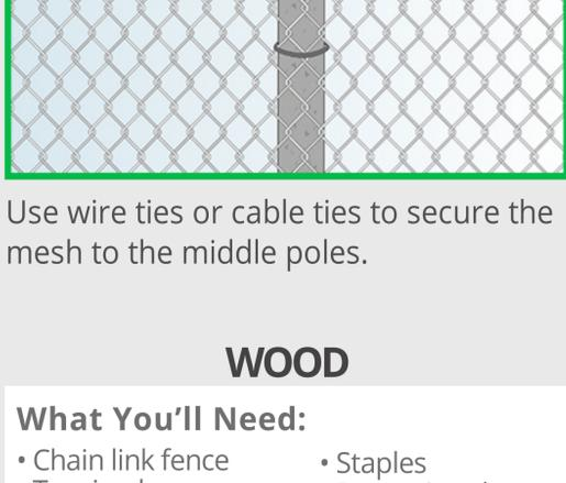
Secure the mesh to the intermediate supports using the same method with fence ties.
