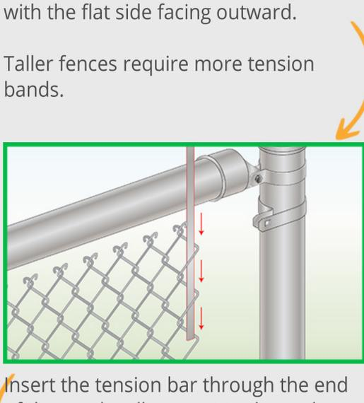
When attaching chain link fence to posts, place tension bands on each post with the flat side facing outward.
