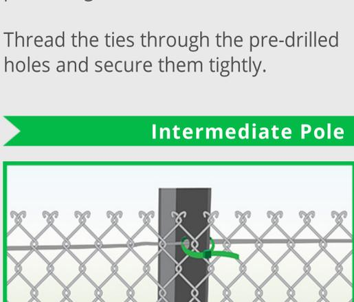
Use wire ties or cable ties to secure the mesh to the middle poles.
