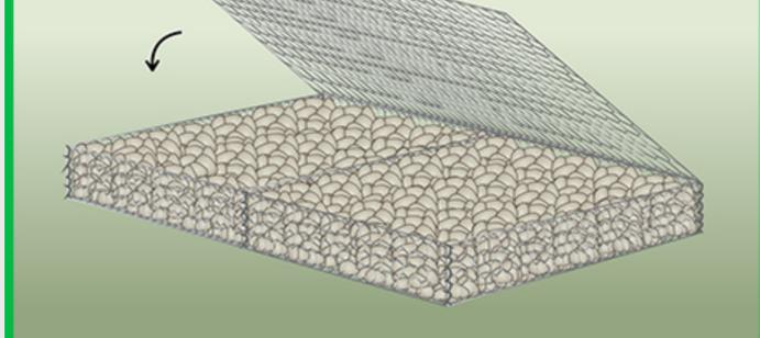
In the process of gabion mattress installation, fold the lid panel over the filled basket, ensuring it fits securely over the stones.
