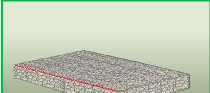
Make sure the lid panels are tightly secured to the gabion mattress by fastening them with tying wire or C-rings, following the same method used for the edges.
