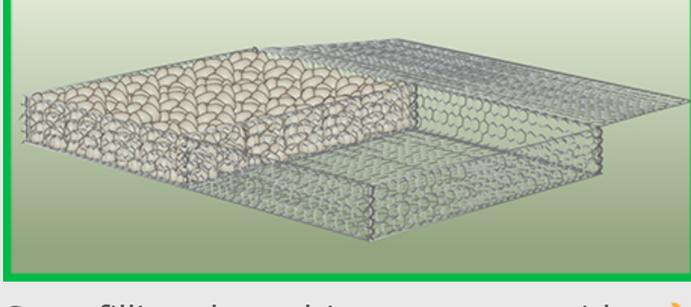
Start filling the gabion mattress with stones of suitable size (minimum 80mm x 80mm).
