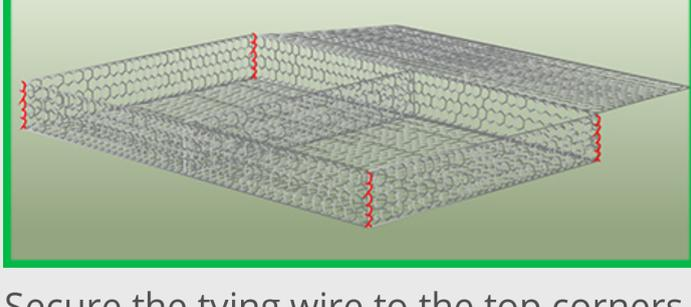
Secure the tying wire to the top corners of the panels, then weave it down along the edges.
