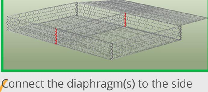
Connect the diaphragm(s) to the side panels and secure them firmly using tying wire.
