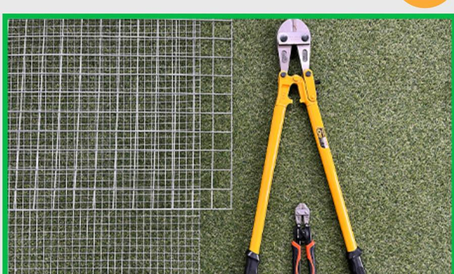
Selecting the appropriate tool primarily depends on the diameter of the wire you need when cutting fence panels.
