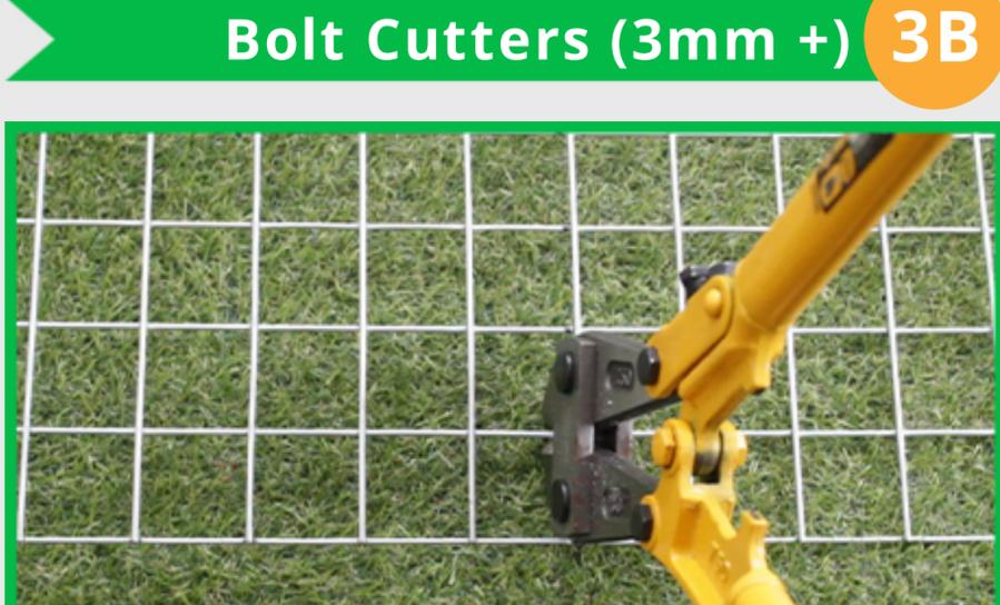
In the process of how to cut a fence panel, the strongest wires can be shortened using a bolt cutter.
