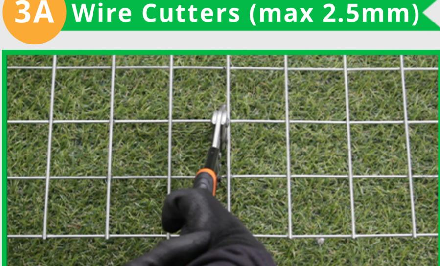
Trim each wire strand individually using a wire cutter, positioning the cuts as close to the weld points as possible.
